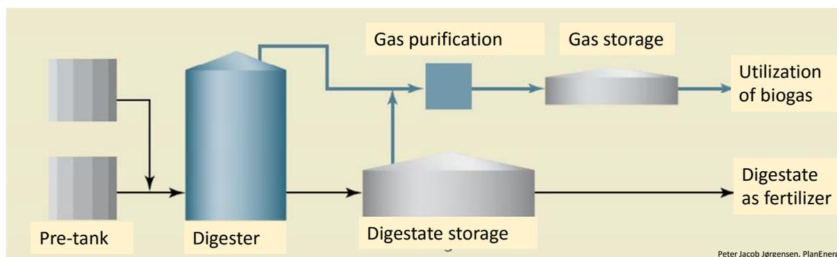
Figure 1. Schematic of biogas plant.
